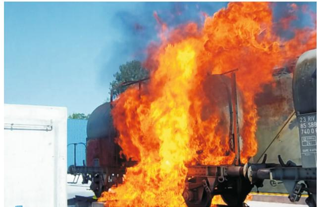
*Fuel Spill below Rail Road Tanker*
