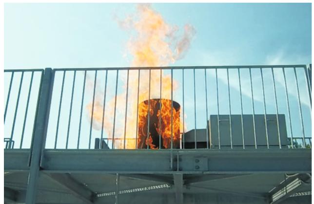
*Overflowing Small Tank Fire*
