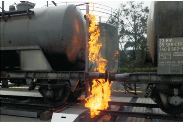
*Rail Road Tanker Leak Fire*
