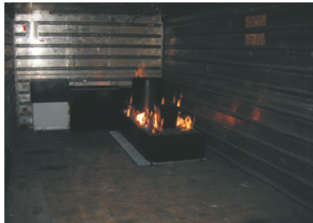
Multi-Prop Fire in Freight Car
