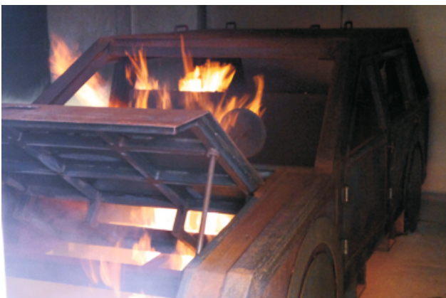
Garage Fire with Car Mock-up
