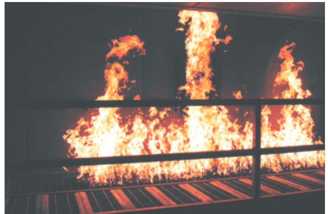
Deck Leaking Flange Fire
