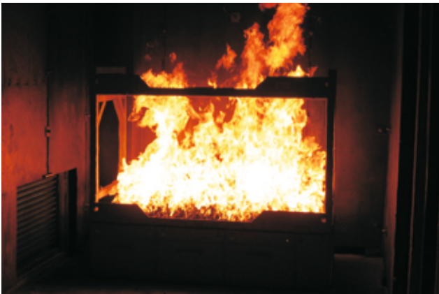
Berthing Mattress Fire
