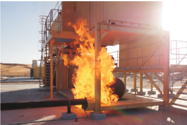
Rupture Tank Spill Fire
