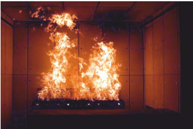
Kitchen Fire With Grease Flare-up
