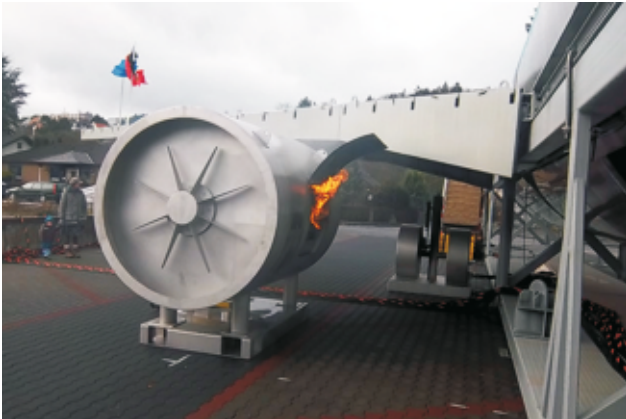
Engine Maintenance Panel Fire
