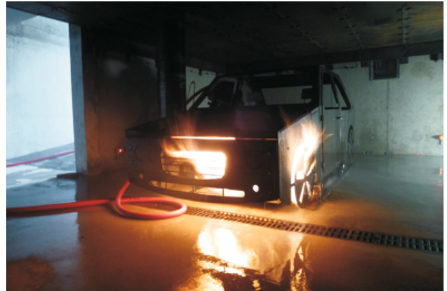
Garage Fire (with Car Mock-up)
