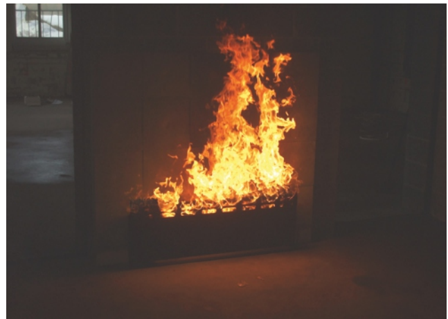
Baseboard "Burn-Through" Heater Fire
