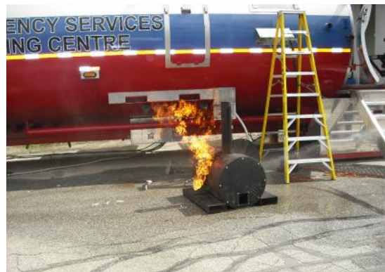
Landing Gear Fire
