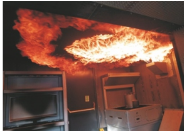
Flashover (Stage 2 of 3, Trainer B)
