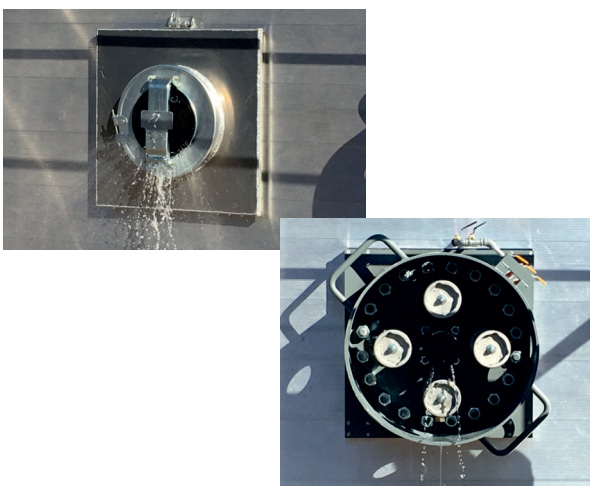
training dome leak simulation
