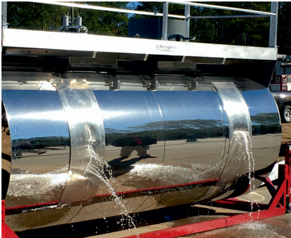
tank fuel leak simulation
