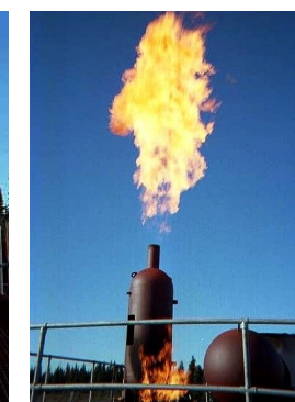
vertical tank fire
