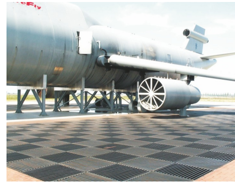
Patented "Drive-On" Fuel Spill allows rescue vehicles to drive right up to the aircraft mockup.
