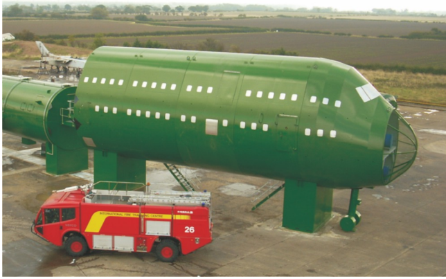
ICAO-compliant aircraft fire training simulator
